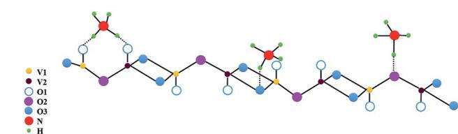
Fig. 11 Adsorption sites for  $NH_3$  adsorption at Brønsted acid sites consisting of singly coordinated, di-coordinated and tri-coordinated oxygen sites on  $V_2O_5$  surface atoms.
