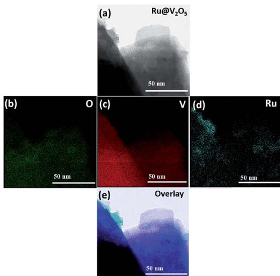
Fig. 4 (a) HAADF-STEM image of an edge portion of a 1%Ru@V<sub>2</sub>O<sub>5</sub> particle (b) elemental mapping of oxygen (c) elemental mapping of vanadium (d) elemental mapping of ruthenium (e) overlay image of oxygen, vanadium and ruthenium.
