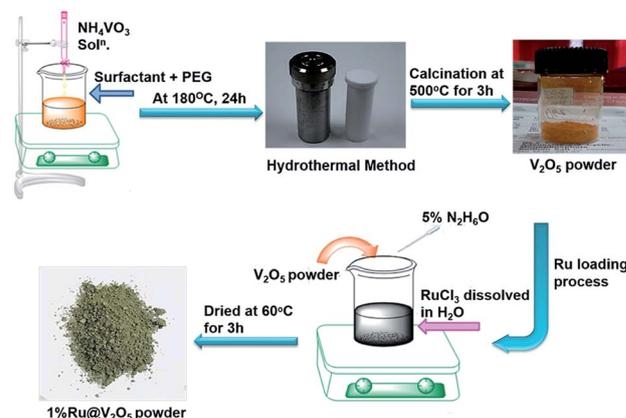
Scheme 1 Schematic representation of  $V_2O_5$  and 1% $Ru@V_2O_5$  synthesis.
