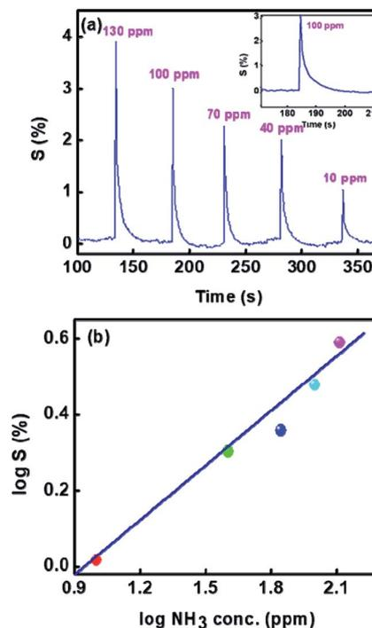
Fig. 9 Sensitivity of  $1\%\text{Ru}@V_2O_5$  (a) as a function of time for various concentrations of  $NH_3$  and (b) log–log plot of sensitivity vs. ammonia concentrations.
