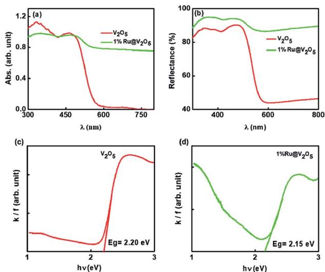
Fig. 5 (a) Optical absorption spectra (b) reflectance spectra (c and d) corresponding  $k/f$  vs.  $h\nu$  Kubelka–Munk plots of V<sub>2</sub>O<sub>5</sub> and 1%Ru@V<sub>2</sub>O<sub>5</sub>.
