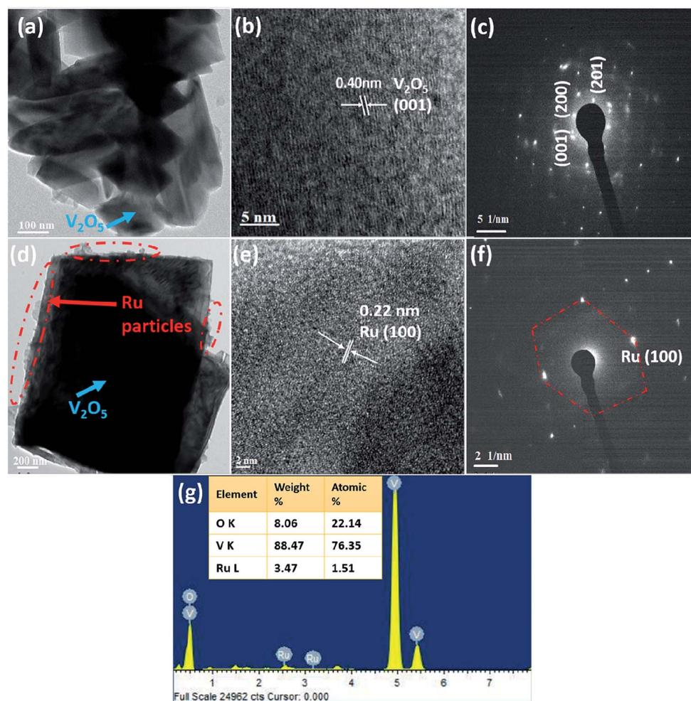
Fig. 3 FE-TEM analysis (a) overview image of  $V_2O_5$  particles (b) lattice resolved image of  $V_2O_5$  (c) electron diffraction of  $V_2O_5$  (d) a single particle of 1%Ru@ $V_2O_5$  (e) lattice resolved image of 1%Ru@ $V_2O_5$  (f) electron diffraction of 1%Ru@ $V_2O_5$  (g) EDAX of 1%Ru@ $V_2O_5$ .
