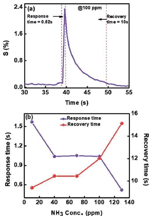
Fig. 10 (a) Dynamic response to  $NH_3$  (b) response and recovery times of 1%Ru@ $V_2O_5$  at 30 °C for different concentrations of  $NH_3$  gas.
