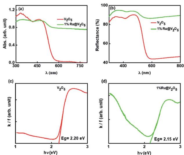
Fig. 5 (a) Optical absorption spectra (b) reflectance spectra (c and d) corresponding  $k/f$  vs.  $h\nu$  Kubelka–Munk plots of V<sub>2</sub>O<sub>5</sub> and 1%Ru@V<sub>2</sub>O<sub>5</sub>.
