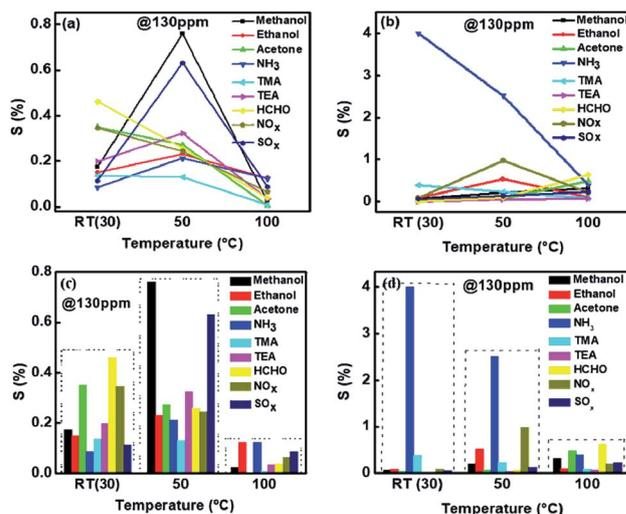
Fig. 6 Comparison of (a) sensitivity of V<sub>2</sub>O<sub>5</sub> and (b) 1%Ru@V<sub>2</sub>O<sub>5</sub> towards different gases. Sensitivity shown as bar graph, at different temperatures, for (c) V<sub>2</sub>O<sub>5</sub> and (d) 1%Ru@V<sub>2</sub>O<sub>5</sub>.
