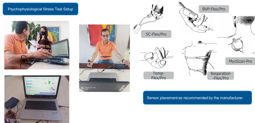
Figure 4. Stress test setup with connected subject on the left, and on the right, sensor placement as recommended by the manufacturer. Images are taken from the ProComp5 Infiniti™ Hardware Manual with the consent of Thought Technology, Montreal, QC, Canada. www.thoughttechnology.com (accessed on 6 December 2021).
