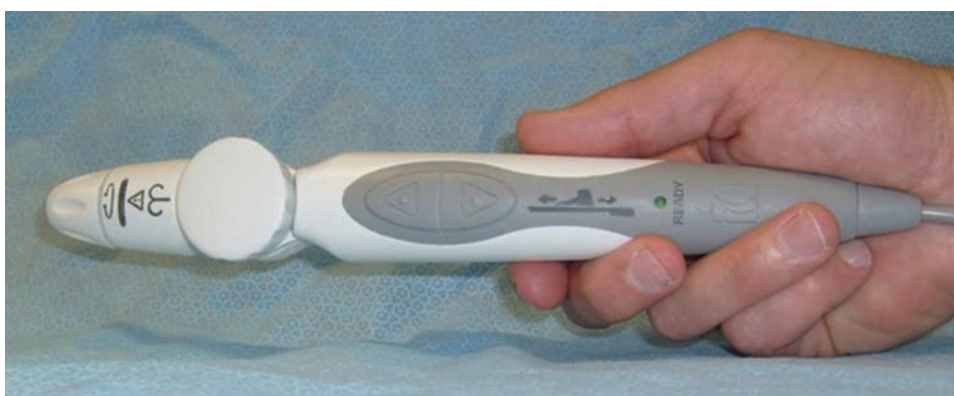
Figure 2: The Amigo™ RCS (Catheter Precision, Inc., Mount Olive, NJ, USA) remote controller. The design resembles a traditional catheter handle and allows for the user to remotely advance, withdraw, rotate and deflect the tip of an attached standard mapping or ablation catheter as desired.
