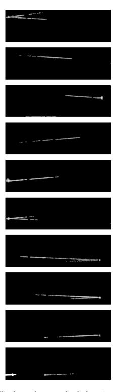
**Figure 3.** Images of the travelling laser pulse captured at the frame interval of 10 ns (from the bottom to the top). Much higher spatial resolution is achieved by the silicon image sensor than most of past light-in-flight imaging, except holographic images by Kubota and Awatsuji [2,3].
