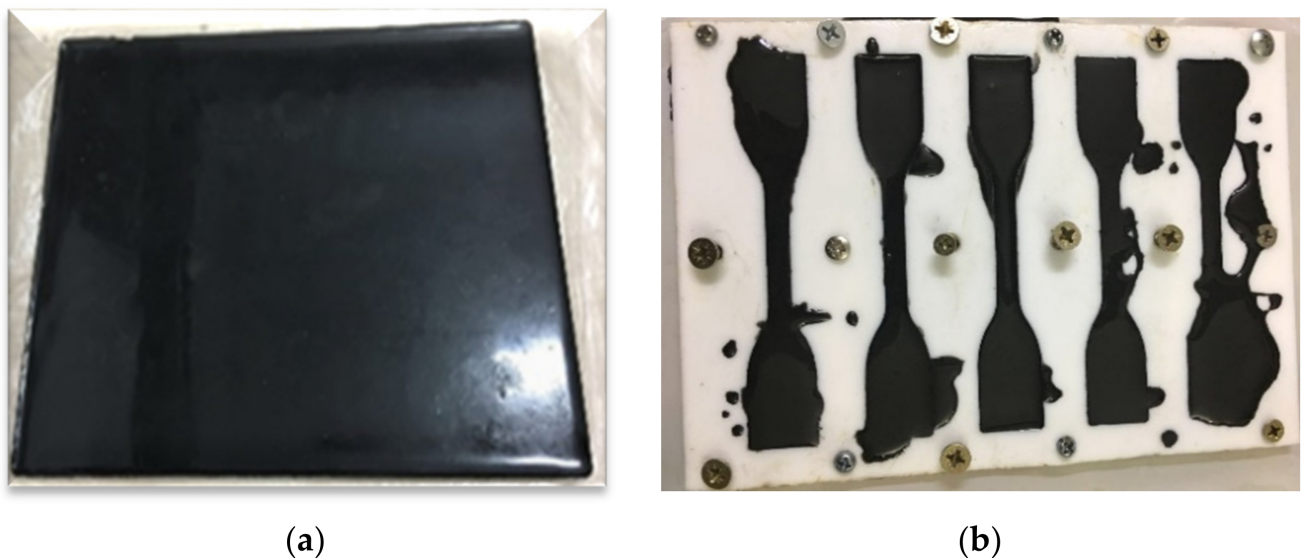
Figure 3. Photographic images of (a) Cured epoxy/CNT nanocomposite and (b) Uncured epoxy/CNT nanocomposite for the tensile tests.
