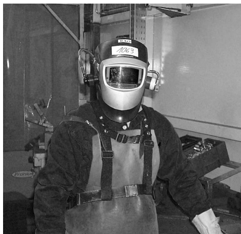
Fig. 1. Welder equipped with the PGP-EA sampler on the right side and the GSP sampler on the left side, both facing inside the shield.
