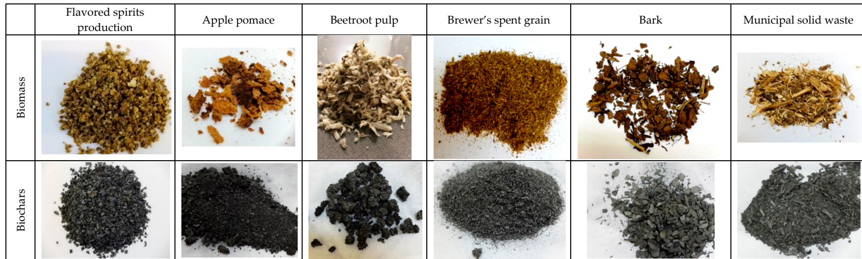
Figure 1. Photographs of the raw and carbonized materials. Thermal decomposition performed under conditions of limited oxygen access with gradually increased temperature up to 850 °C over 30 min and continued for 60 min at a constant temperature.
