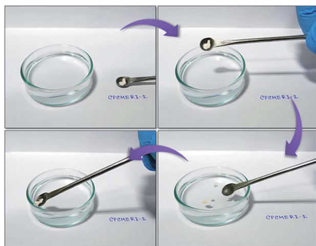
Fig. 12 Hydrophobic behaviour of CPCMERI-2 over water surface.
