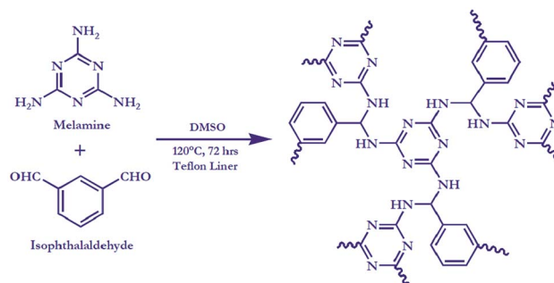
Scheme 1 Schematic representation of the synthesis of CPCMERI-2 .
