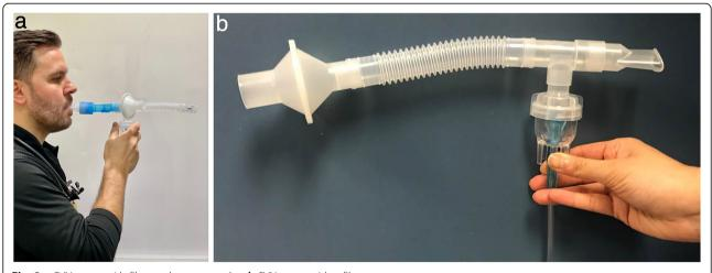
Fig. 3 a SVN setup with filter and one-way valve.  ${\bf b}$  SVN setup with a filter
