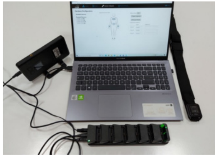
Figure 1. Mobility Lab System: access point, docking station, movement monitor, Mobility Lab software.
