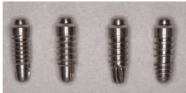
Figure 1. The custom-made dental implants used in this study. The thread shapes, from left to right, are V-shaped, buttress, reverse buttress, and trapezoid.
