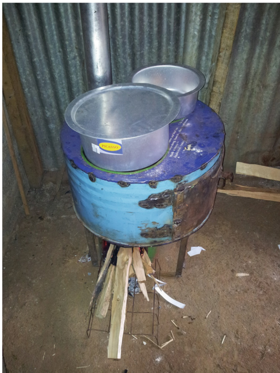
Figure 5 Locally constructed, improved cookstove installed in Kenya.
