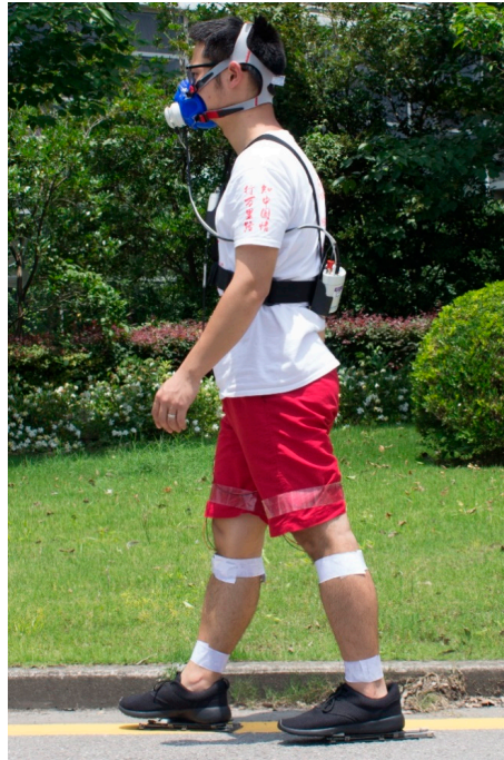
Figure 2. Experimental setup. Subjects performed 200 m normal and fast walking trials on flat ground with the custom sliding shoes. Metabolic rate was measured with a portable breathing analysis system and energy harvesting rate was measured from the generator on the custom sliding shoes.
