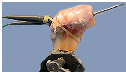
Figure 1. Ox-bone model ready for peripheral reaming and temperature measurement.
