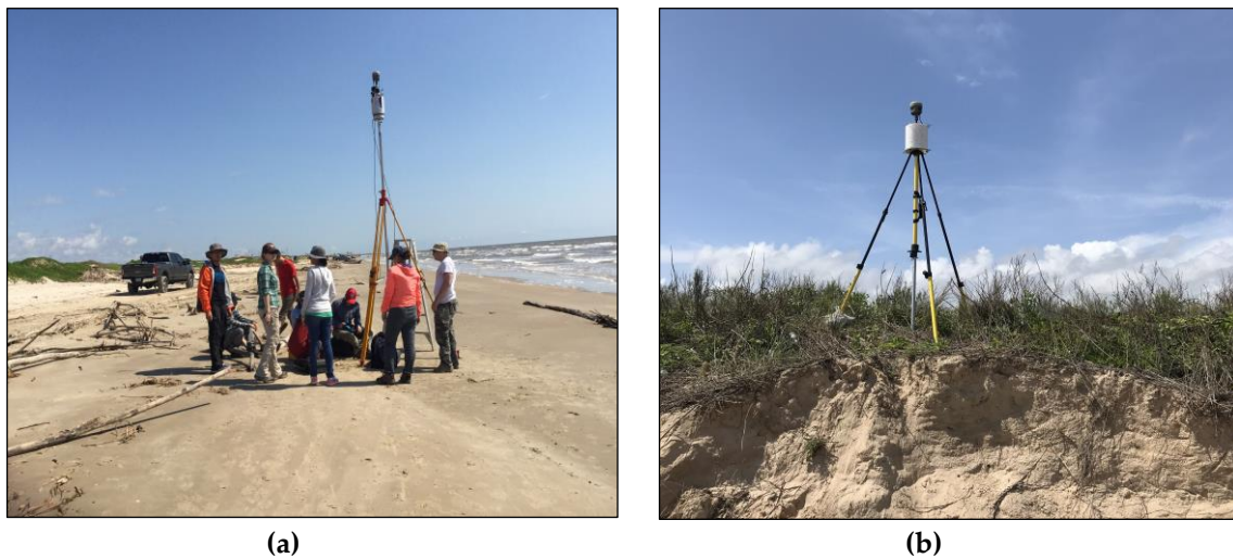
Figure 6. Photos showing field equipment used by the rapid TLS surveying method in the field. (a) A Riegl VZ-2000 scanner with a co-mounted Trimble R10 GPS unit; (b) a cylinder reflector with a co-mounted Trimble R10 GPS unit.
