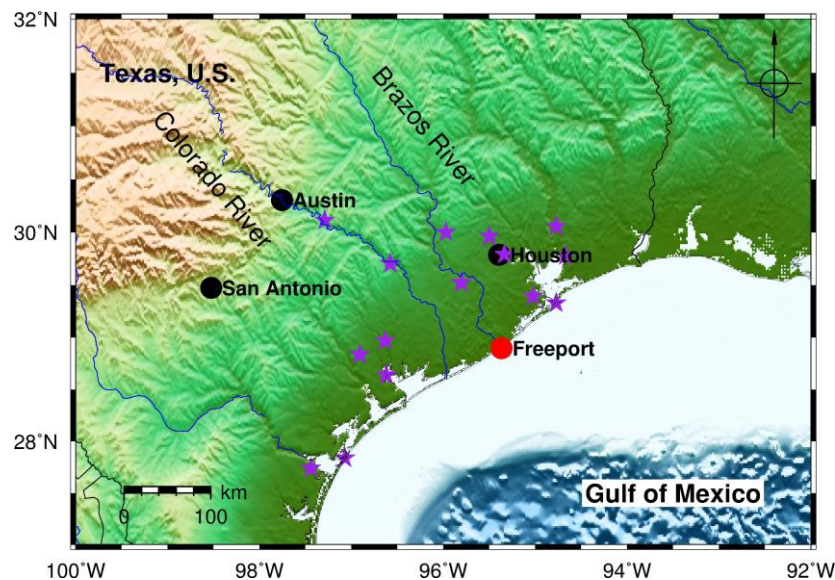
Figure 1. Map showing the location of the study area in Freeport, Texas, USA. Purple stars represent Continuously Operating Reference Stations (CORS) used by the Online Positioning User Service (OPUS) for solving the positions of the scanner according to 15 to 30-min static GPS observations.
