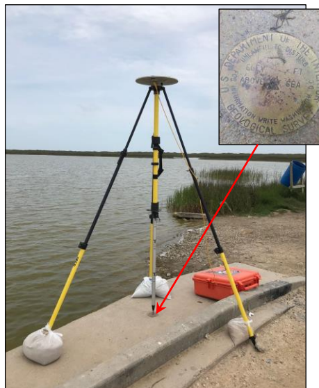
Figure 7. A photo showing the U.S. Geological Survey (USGS) permanent benchmark and the setting up of a reference station for kinematic GPS mapping in the beach area.
