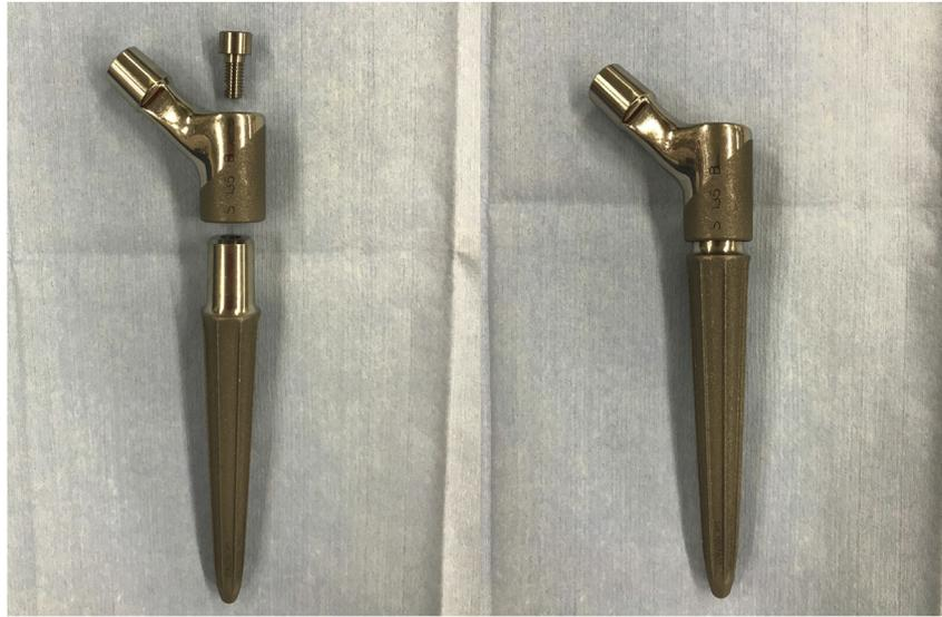
**Figure 1.** The MODULUS stem system. This stem system is comprised of a stem and a neck. The stem has a rough blasted surface and radial fins. The neck part can be inserted into the stem at any version and fixed by taper lock and screw.
