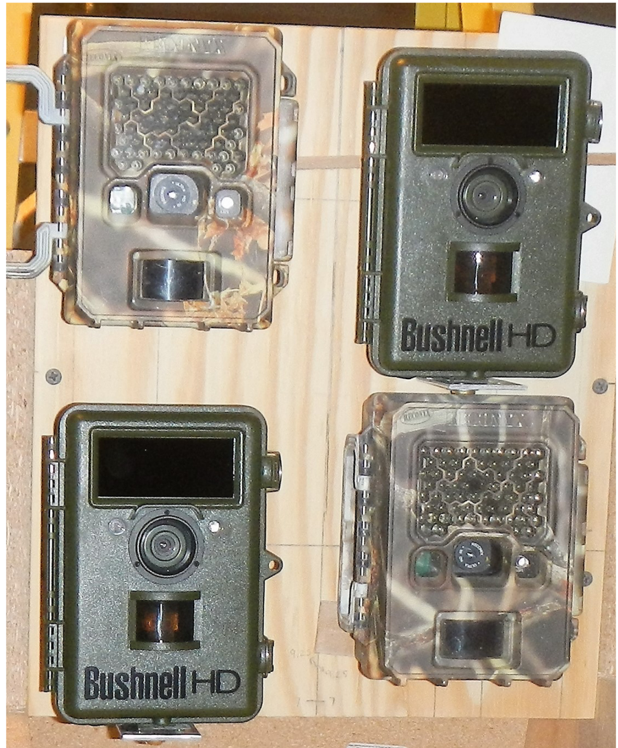
Fig 2. Experimental and Control cameras (B1, R1, B2, R2) aligned to center of backdrop.
