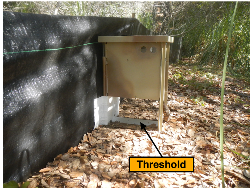
Fig 4. Drift fence with camera trap box. Camera inside locked box with battery and mounted vertically above HALT threshold.
