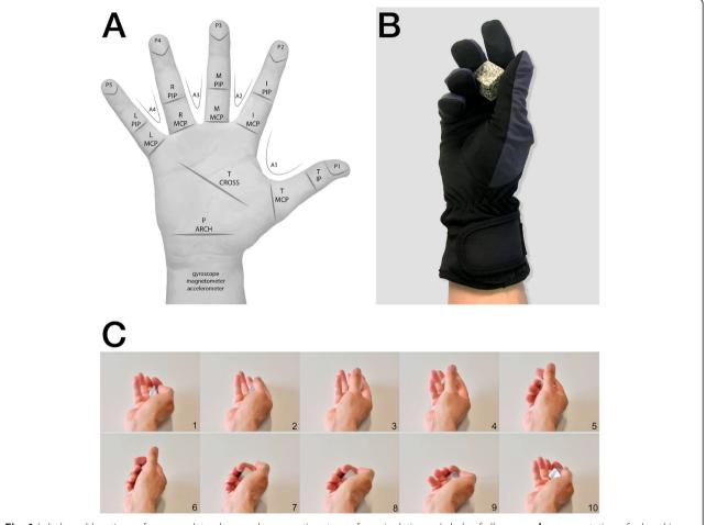
**Fig. 1** Labels and locations of sensors, data glove and consecutive steps of manipulation. **a** Labels of all sensors, **b** representation of a hand in the data glove holding the cuboid, **c** image sequence of instruction video showing manipulation of cuboid (one motor act)
