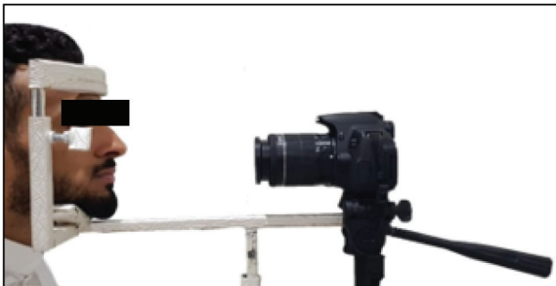
Figure 1: A special device was constructed to standardize the distance from the camera to the teeth
