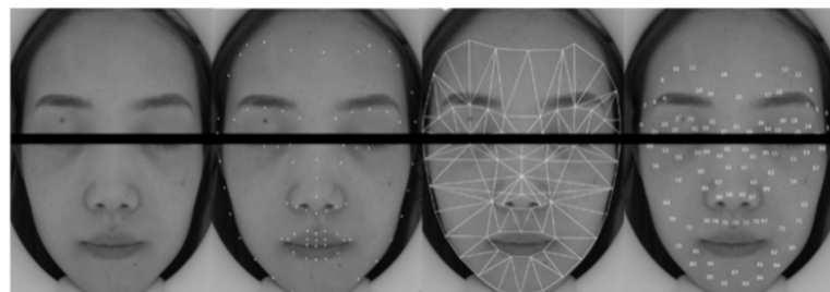
Figure 5. Facial landmarks detection and ROI extraction. Left two are the original image taken by the camera and the 81 facial features detected. Right two represent the 98 triangular regions formed by combinations of different landmarks and the number of each triangular region.
