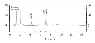
FIGURE 1: Chromatogram of plasma sample containing  $4.00 \ \mu g/mL$  of internal standard (IS, retention time =  $4.217 \ min$ ) and  $4.00 \ \mu g/mL$  of caffeine (retention time =  $7.082 \ min$ ).
