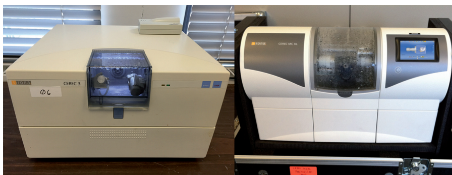
Fig. 1. Milling CAD/CAM units used in this study: Cerec 3 (left) and Cerec MXCL Premium Package (right).
