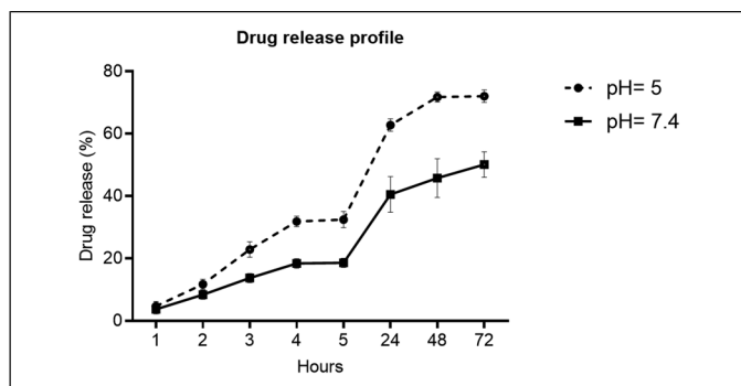
Figure 3. The drug release profile of PEG-CS-FA-Sb nano-complex at pH values of 7.4 and 5.0. Nanocarrier indicates a controlled Sb release behavior at physiologic pH (7.4) than acidified pH (5.0). The main cause of release in acidified pH is the protonation of the CS chains which results in a fast Sb release ratio. This fast drug release is significantly suitable for cancer therapy since the environments of cancer cells and as well as endosomal organelles are acidified. Abbreviations: CS, chitosan; PEG, polyethylene glycol; Sb, sodium butyrate; FA, folic acid.
