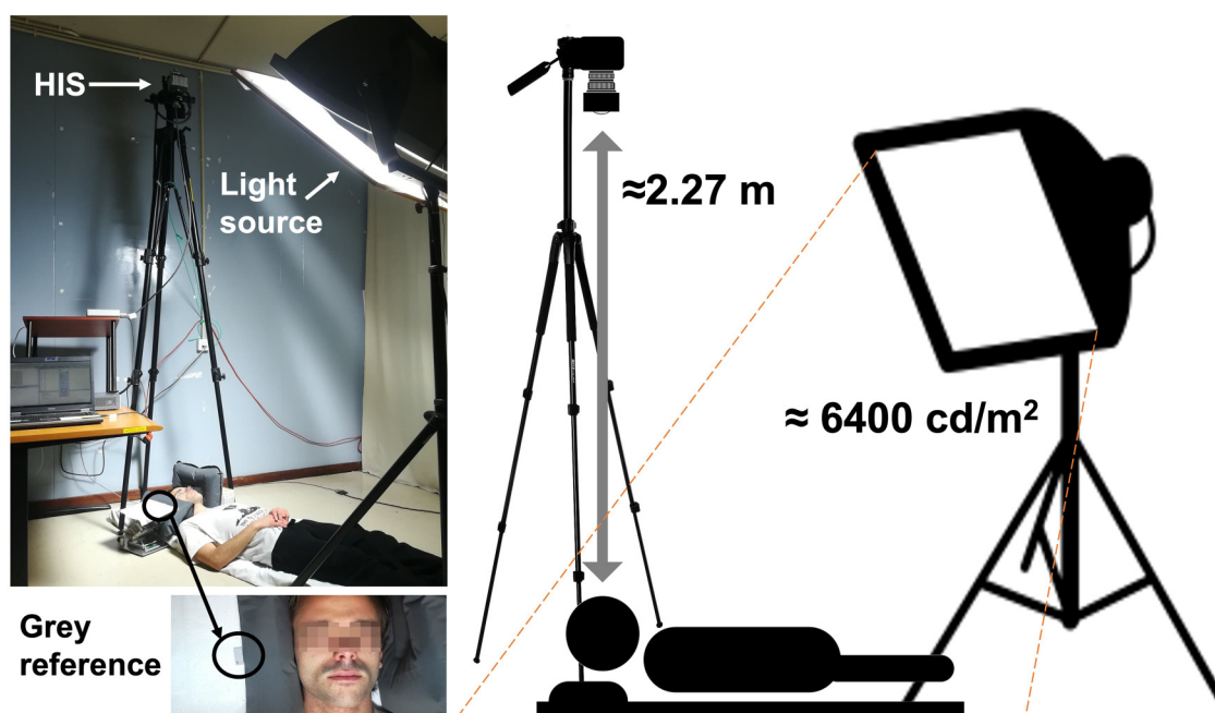
Figure 2. Setup for the acquisition of the hyperspectral images, highlighting the positions of the participant, the camera, and the light source with the UV filter in front. The participant was lying on the floor and the participant's head was supported by pillows. The image's inset highlights the gray reference that was placed at the face level, visible during the time of acquisition.
