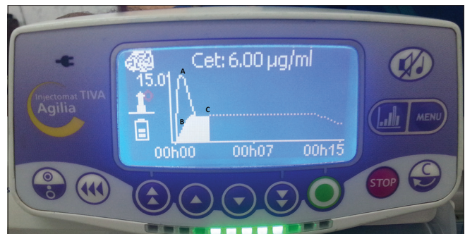
Figure 1: Target controlled infusion pump showing equilibration between plasma concentration and effect concentration. A: Plasma concentration, B: Effect-site concentration, C: Target effect-site concentration
