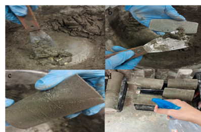
Figure 18. Specimen preparation. (a) Mixing microcapsules with a cement mortar; (b) application of a mixed mortar; (c) rock specimen injected with a microencapsulated mortar; and (d) maintenance process.
