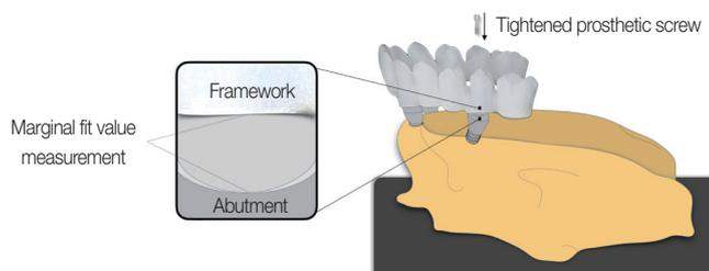
**Fig. 4.** Schematic representation of single-screw test. Prosthetic screw is tightened in the abutment located on the opposite side (abutment D). The marginal fit value measurement is obtained at the framework/abutment interface on buccal side (enlarged view on the left). Values of all abutments (A, B, C, and D) were assessed on both buccal and lingual sides.
