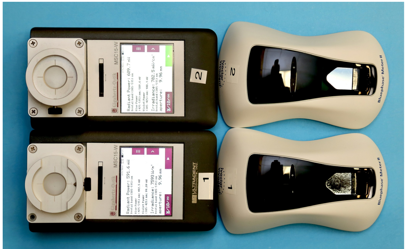
Fig 2. The two examples of the Bluephase Meter II and the Mini Gig radiometer used in the study.
