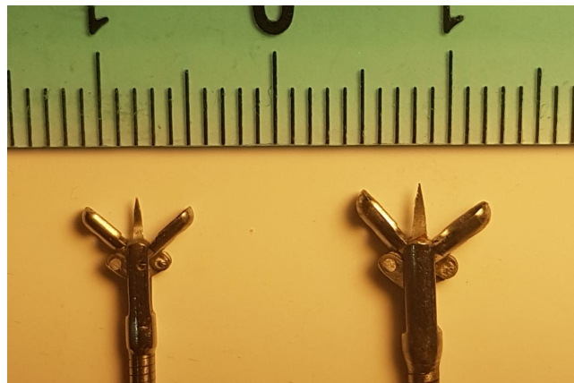
FIGURE 1 Comparison of the dimensions of the smaller (left, 1.8 mm) and larger (right, 2.4 mm) biopsy forceps
