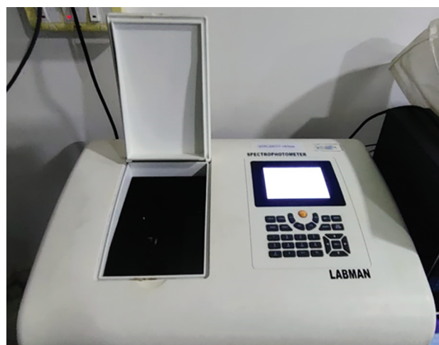
Fig. 2: Spectrophotometer for estimation of protease activity in saliva
