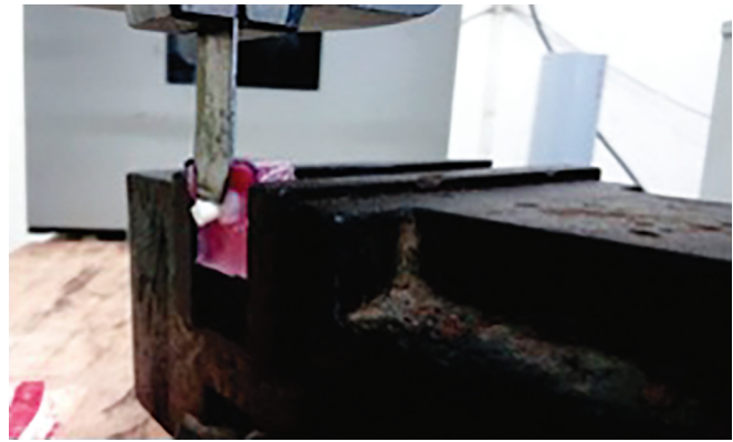
Fig. 4: Testing of shear bond strength
