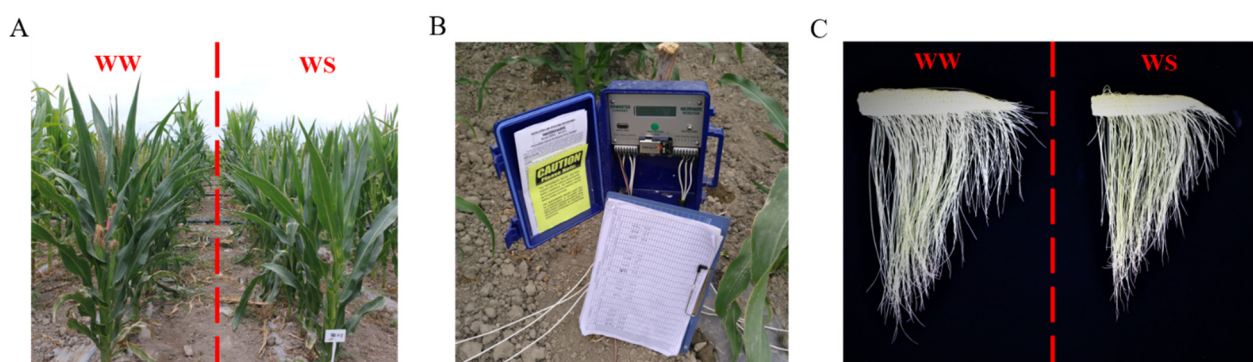
Figure 1. Soil moisture monitor and plant performance under different water treatment: (A) WATERMARK MONITOR installed in the field and connected to the sensor; (B,C) plant height and ear development of drought-sensitive lines under WW and WS condition.
