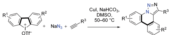
Scheme 12. Cu I -catalysed azidation and click reaction to afford phenanthridines.
