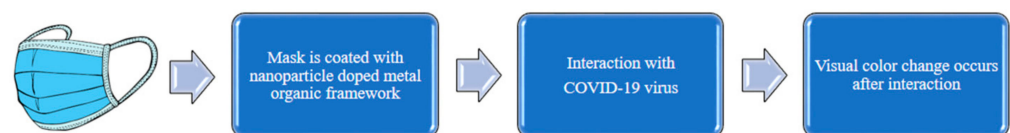
Figure 10. Workflow of a wearable nanobiosensor.
