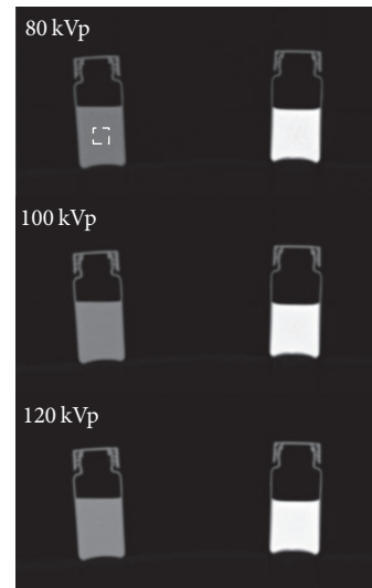
FIGURE 1: CT images of the water vial (left column) and the cortical bone equivalent phantom (right column) at 80, 100, and 120 kVp. A 30 \text{ mm} \times 30 \text{ mm} ROI was drawn in the center of vials. The average CT numbers were taken as \text{CTN}_{\text{mar}} and \text{CTN}_{\text{cor}} for the TCM method.
