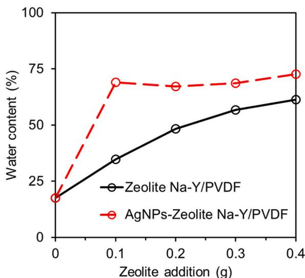
Fig. 4. The effect of zeolite addition on water content of Zeolite Na-Y/PVDF membrane and AgNPs-Zeolite Na-Y/PVDF membrane.
