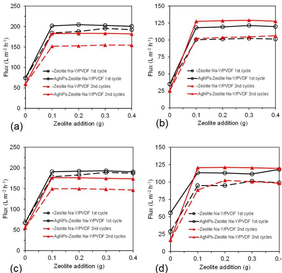
Fig. 3. Flux performance of hollow fiber membrane using water (a) and wastewater (b) as a feed, and flat sheet membrane using water (c) and wastewater (d) as a feed.
