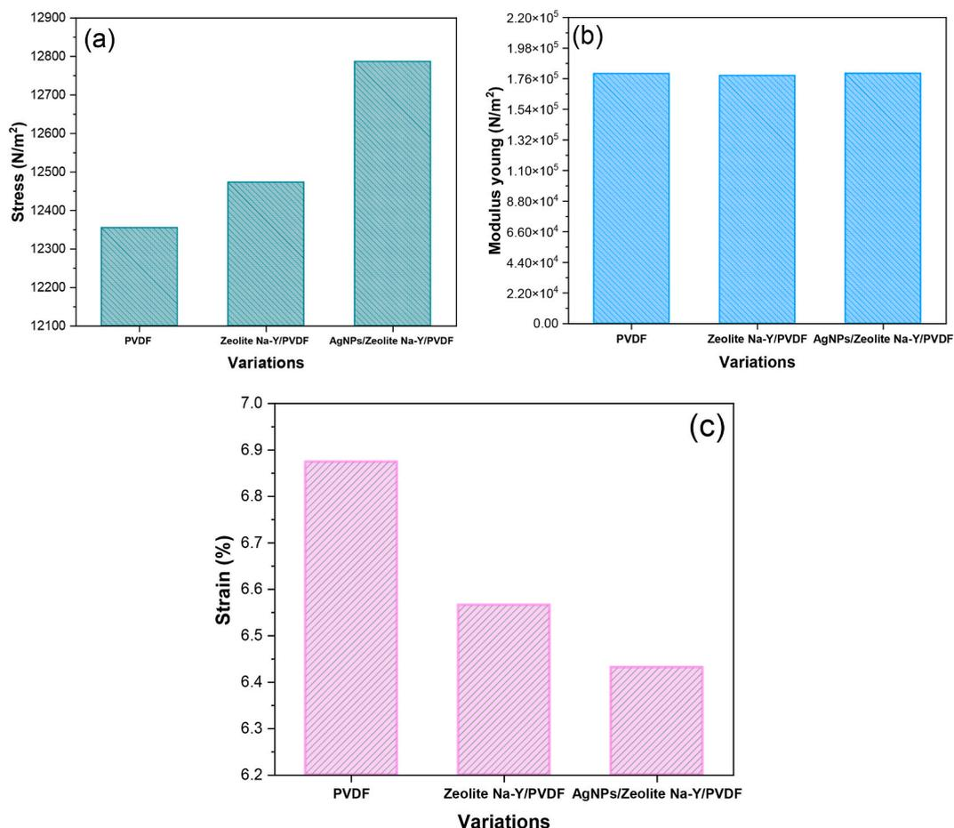
Fig. 2. (a) Stress, (b) modulus young, and (c) strain testing of the membrane.
