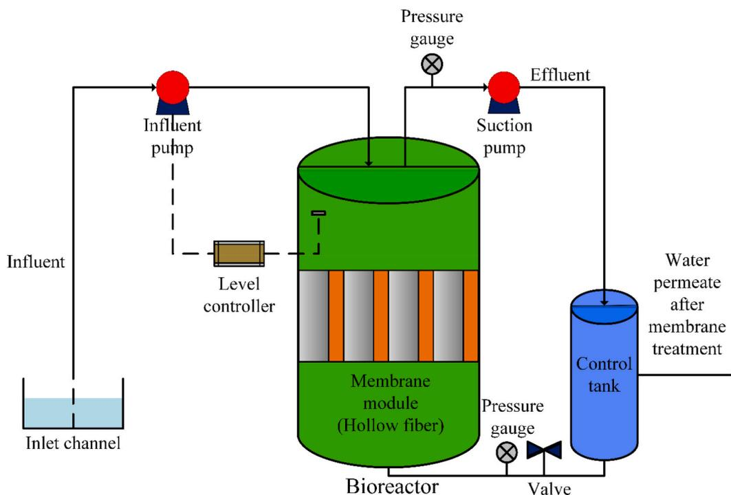
Fig. 1. Ultrafiltration reactor configuration.
