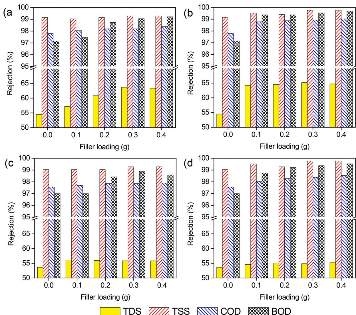
**Fig. 6.** Rejection performance of hollow fiber PVDF membrane with addition (a) zeolite Na-Y (b) AgNPs-zeolite Na-Y, and flat sheet PVDF membrane with addition (c) zeolite Na-Y (d) AgNPs-zeolite Na-Y.
