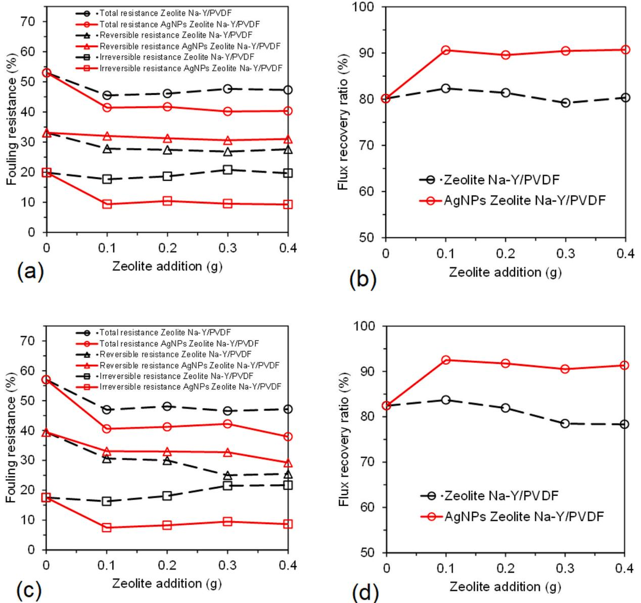
Fig. 5. Antifouling performance a) Zeolite Na-Y hollow fiber membrane, b) AgNPs-Zeolite Na-Y/PVDF hollow fiber membrane, c) Na-Y Zeolite flat sheet membrane, d) AgNPs- NaY/PVDF flat sheet membrane.
