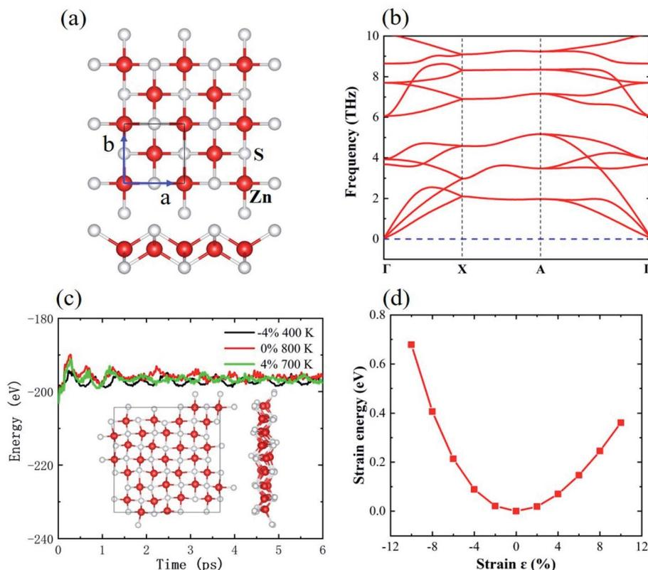
Fig. 1 (a) Top and side views, (b) phonon band dispersion, (c) evolution of total energies with time in the AIMD process under different strains, and (d) strain energy–strain curve of monolayer ZnS.
