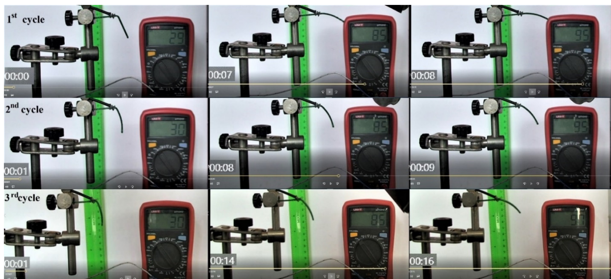
Figure 4. Typical images recorded during the occurrence of free-recovery SME at a 3D printed R-PET specimen during three consecutive heating-cooling-bending cycles. Time duration details (s).
