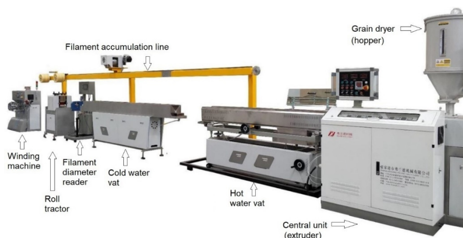
Figure 1. The experimental line for filament production from R-PET grains.
