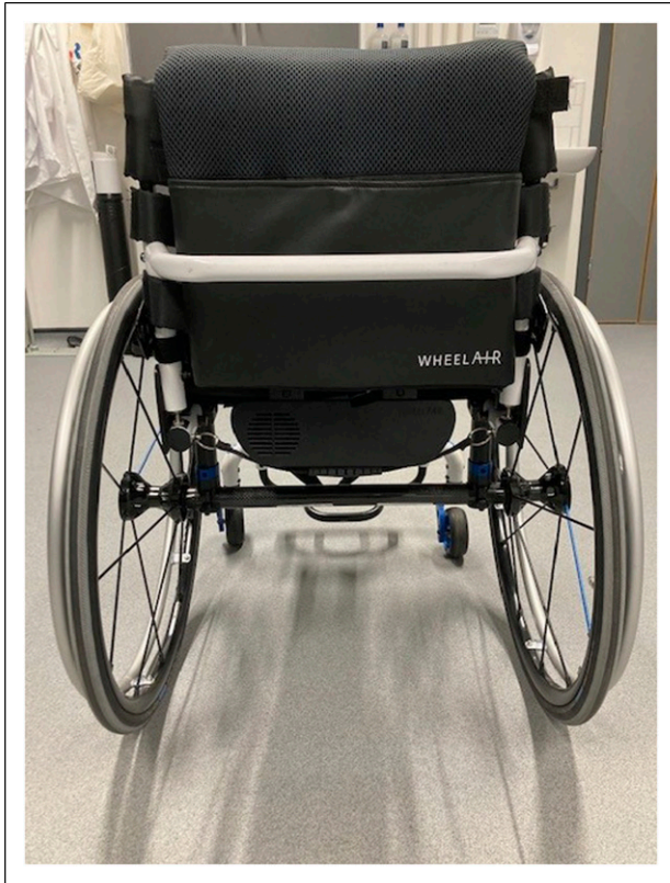
Figure 2. Integrated fan cooling system (WheelAir® slingback) fitted to daily wheelchair.
