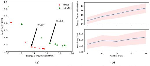
**Figure 4.** Energy consumption and mean delay performance with MILP solver: (**a**) the tradeoff between these two KPIs; (**b**) impact of increasing number of UEs.
