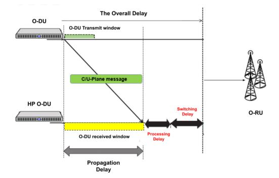
Figure 2. The overall delay in the network.
