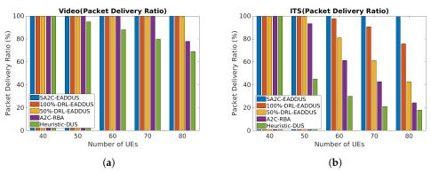
**Figure 7.** The overall packet delivery ratio by considering different processing capacity levels and algorithms: (**a**) the video packets' delivery ratio; (**b**) the ITS packets' delivery ratio.
