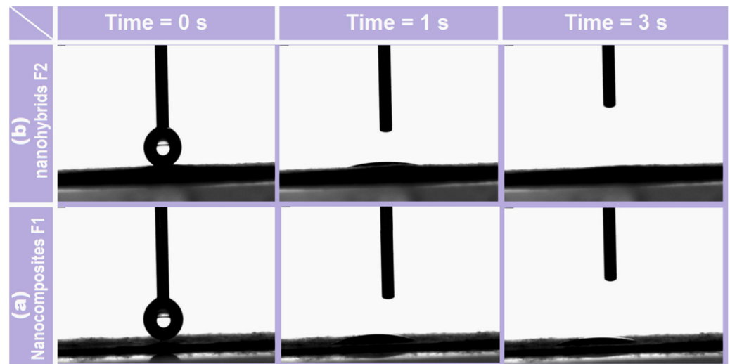
Figure 7. Water contact angle experimental results: (a) electrospun core–shell nanohybrids; (b) electrospun nanocomposites.
