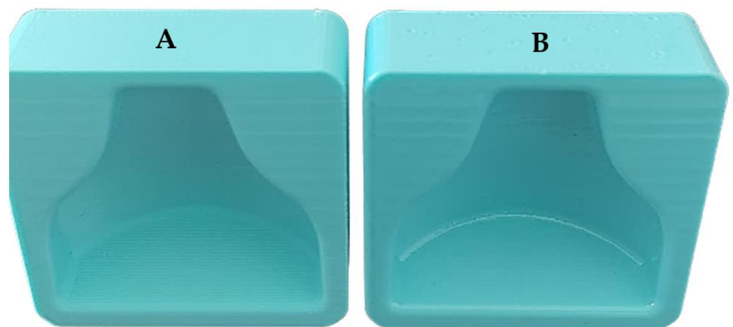
Figure 6. (A) Mold immediately after printing; (B) mold after smoothing treatment. On the top of the (B) mold are small circular spots; these are due to the support surface during smoothing and the rotation of 180 degrees. In the lower part of the mold (A) it is possible to see the layers, due to the staircase effect; on the right they have disappeared thanks to the smoothing process.
