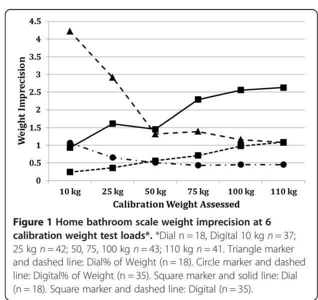
**Figure 1** Home bathroom scale weight imprecision at 6 calibration weight test loads\*. \*Dial n = 18, Digital 10 kg n = 37; 25 kg n = 42; 50, 75, 100 kg n = 43; 110 kg n = 41. Triangle marker and dashed line: Dial% of Weight (n = 18). Circle marker and dashed line: Digital% of Weight (n = 35). Square marker and solid line: Dial (n = 18). Square marker and dashed line: Digital (n = 35).
