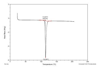
Fig. 1. DSC analysis of 3-o-ethyl-l-ascorbic acid.
