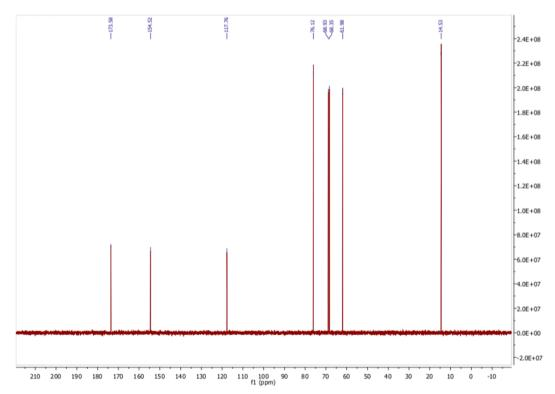
Fig. 4. <sup>13</sup>C NMR spectrum of 3-o-ethyl-l-ascorbic acid in D<sub>2</sub>O.
