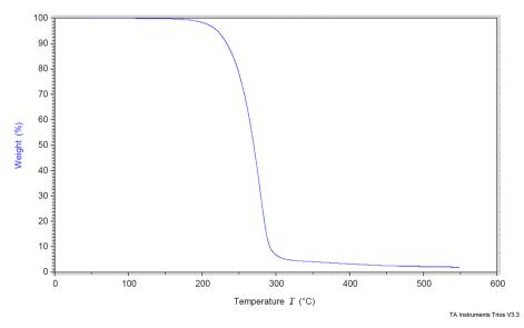
Fig. 2. TGA analysis of 3-o-ethyl-l-ascorbic acid.
