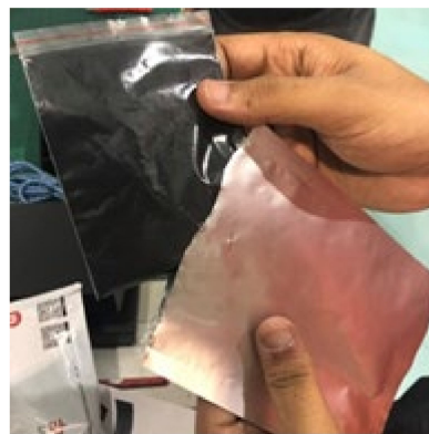
Figure 1. Helical multiwalled carbon nanotubes (HMWCNTs) used in the experimental work.
