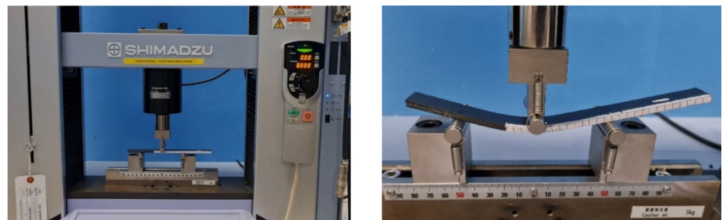
Figure 6. Experimental set up for the ENF specimen.
