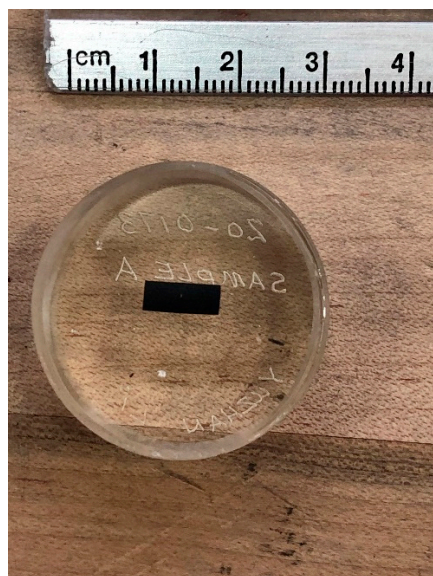
Figure 2. The as-received polymer nanoindentation sample that was cold mounted in epoxy and polished to a mirror finish.
