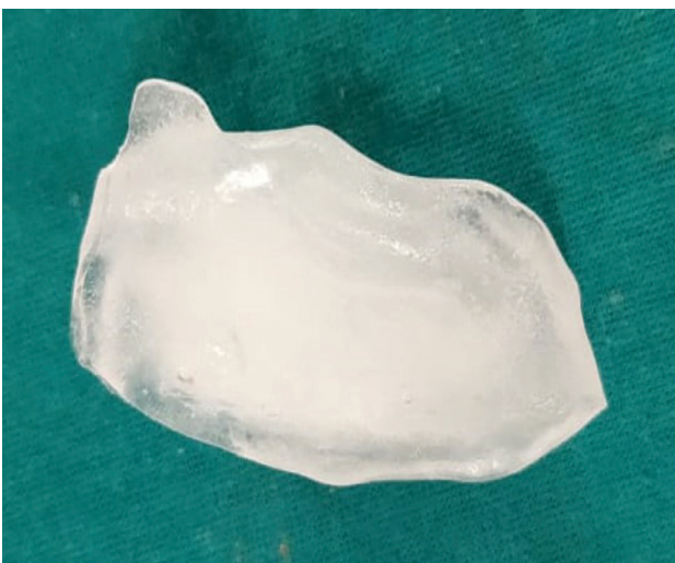
Figure 7. Ice block retrieved from the wax pattern.
