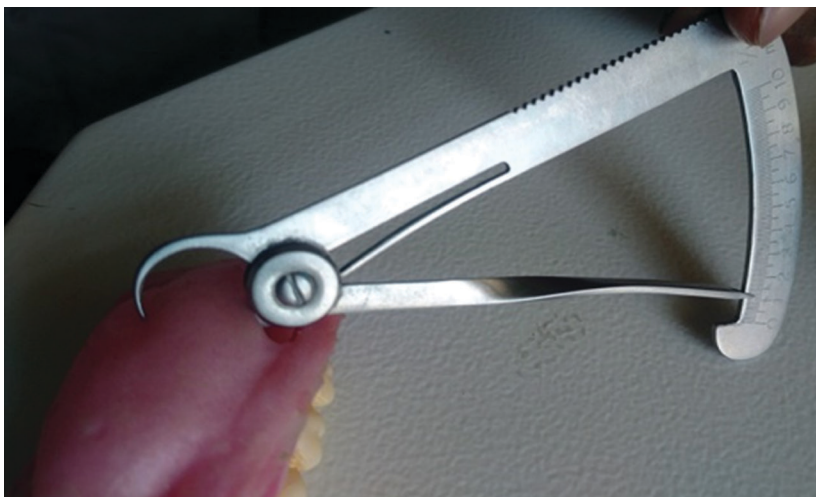
Figure 11. Uniform thickness of the prosthesis measured using a vernier caliper.
