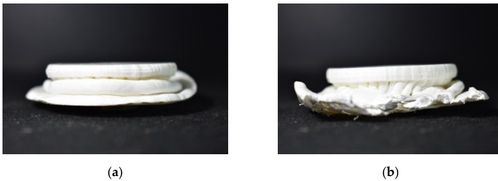
Figure 20. (a) Compressed model; (b) Failed model while testing.
