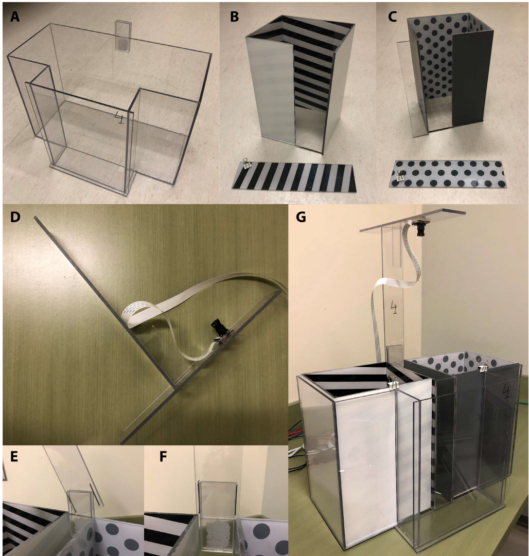
Fig. 2. Illustrative images of the CPP box. The main body of the box (A) consists of a single large compartment which accommodates two smaller compartments with distinct contextual cues and removable doors (B,C). A removable arm is holding the camera for recording of behaviour (D). The arm slots in between two polycarbonate pieces attached to the back of the main body (E,F). During conditioning, the patterned compartments are closed off (G), but remain opened during the CPP test phase.
