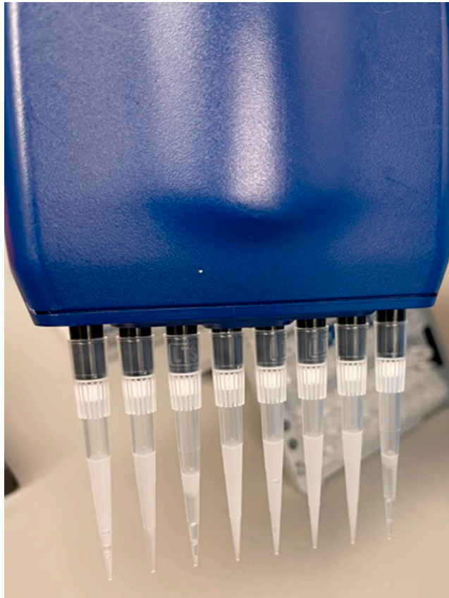
Figure 2. Tips 3 and 8 are not homogeneous and have an excess of partitioning oil, indicating a clog The other tips are successfully generated GEM emulsions.
